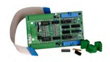
The XIOM is a 16 way universal input/output expansion board. The I/O on the XIOM can be set in banks of 8 to operate as follows:
