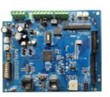
The MPM801 NexGen Multi-Purpose Interface Module is used to interface between the controller and the expansion modules through the Remote Bus. The MPM801 module is compatible with the legacy MPM800 module, except that the MPM801 module does not include the LCD or the keyboard interface. The MPM801 module provides remote connection over the new X-Bus for zonal displays such as the FCZ4DS, and FCZ8DS. The X-Bus also supports the ANN820, ANN840, and the ANN880.
