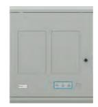
The FireClass FC-EAS Evacuation Alert System is an addressable panel that uses FC600 technology. It can have four standard power loops or two high-power loops, and each panel can have a maximum of 500 addresses. This provides the flexibility to allocate all available power, and 250 addresses, to the high-power loop, or to share resources across two shared power loops. The panel has a shallow housing that can accommodate batteries with a maximum capacity of up
