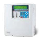
Triple Circuit single loop panel, supporting up to 128 loop devices. The overlay has icons, this makes the panel suitable for all markets. 1,5A power supply unit.
